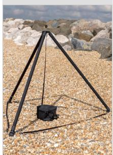
**9.** Peg down the feet using the rock pegs or (if on concrete) place sandbags over the feet
