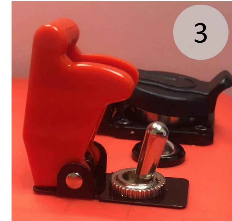
Arming switch exposed prior to switching to the on position.
