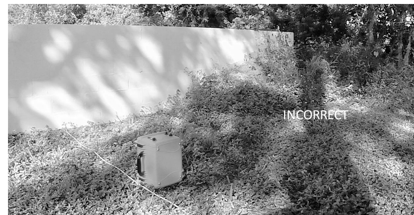
FIGURE 3-15 sensor too close to a cinder block wall.
