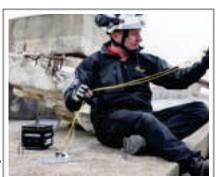
The WASP Multi-Purpose Plate can then be lowered ore slid into position using the WASP Carabiner Slip Lock. The end away from the plate can be secured via a carabiner to a suitable anchor. The unit should be set prior to lowering.
