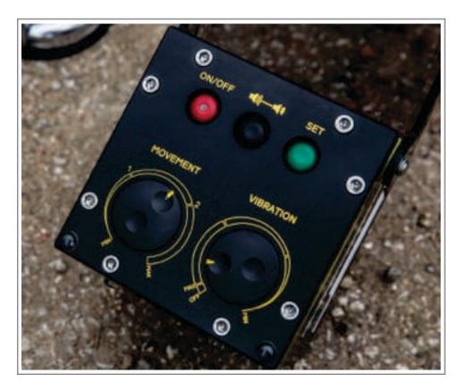
Alarm the WASP using three push buttons and two rotary dials
