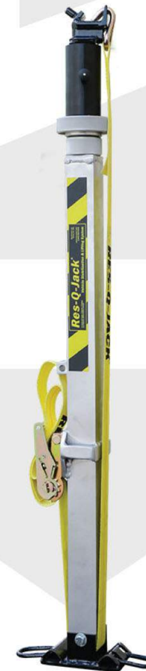
LONG STRUT ATX-STRT-L The standard-length Auto X is a light-weight, easily portable, all-in-one strut for light-duty rescue scenarios. Comes standard with our Swivel CRG end fitting and built-in Ratchet Strap with Wire Hooks. (Extensions are not permitted on standard size strut). Height Extended: 87.25" / Collapsed: 54.5"
