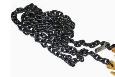
GRADE 80 CHAIN ACC-CHAN | 16' ACC-CHAN-20 | 20' This rugged chain is 3/8" with grab hooks and a WLL of 7100 lbs., this chain is approved for overhead lifting. Available in 16' or 20' lengths.
